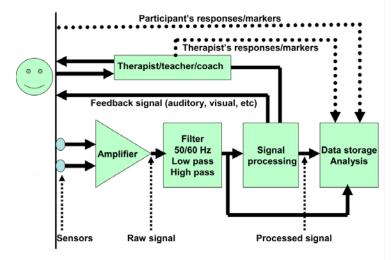
*Figure 1*. Flow diagram of biofeedback equipment in which the signal is recorded from the person, amplified, processed, stored for later retrieval and analysis, and transformed into a signal that is fed back to the participant. In many cases, the therapist/coach/trainer can be the intermediary for the feedback signal. In addition, the participant's responses can be collected, analyzed, and correlated to the recorded physiological signals. By permission from Peper et al., (2009).
